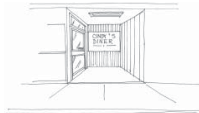
Poorly altered entryway: door relocation, modern door with no windows.
