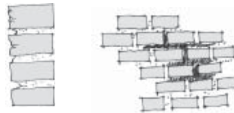
Tuck point brick walls when water infiltration is occurring or pockets in the mortar have formed (see graphic above). Tuck pointing is simply reapplying mortar to the joints between bricks, as pictured below.
